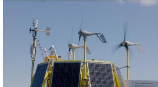
Various configurations are possible, depending on wave conditions and local weather, for instance. As specifications vary from one project to another, its design is modular and easily adaptable, supporting a wide range of metocean and environmental sensors.
