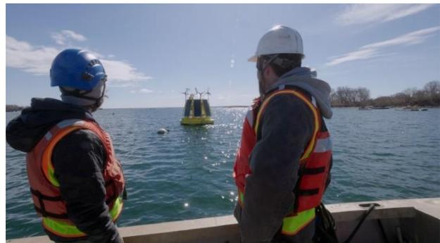
CLS Group DeepCLiDAR buoy systems are now available to the offshore wind market to provide robust, accurate, harsh environment, eco-friendly, wind resource and metocean
