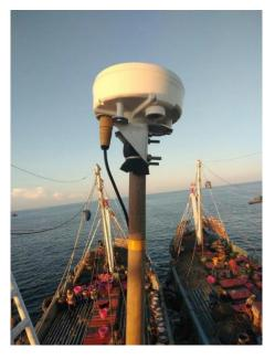
The Triton Advanced Terminal is one of the world's leading Vessel Monitoring Systems (VMS) terminals. It automatically transmits the position, speed, heading and logbook via satellite. It is robust, highly reliable and easy-to-install.
