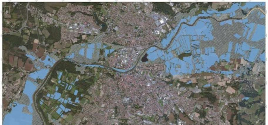
**Since 2013**, CLS and its subsidiary ALTAMIRA INFORMATION, have been mapping and delimiting flood zones of the Adour river in Dax, using their expertise in satellites and radar imaging.
