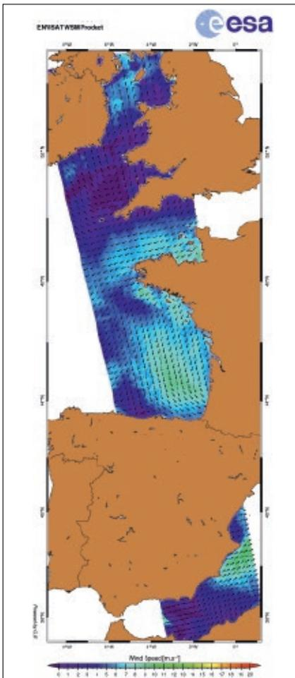
**Satellite radar images processed by CLS** provide high resolution wind strength and direction information. ©CLS/ESA
