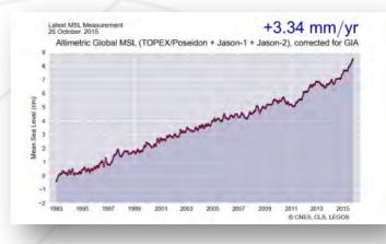
based on space altimetry data from several satellites. The "sea level" indicator calculated by CLS is increasingly reliable and more and more accurate. It is no doubt one of the best products available today. This will be even more true with the data from Sentinel-3.
