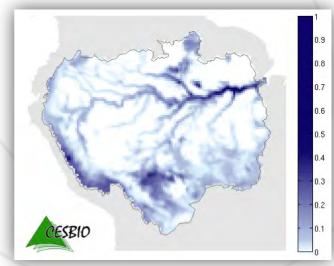
Estimate of open water areas seen by SMOS between 2010 and 2015. These will be coupled with altimetry data (JASON-2, JASON-3, Sentinel -3) to obtain the volumes of water in the Amazon Basin.
